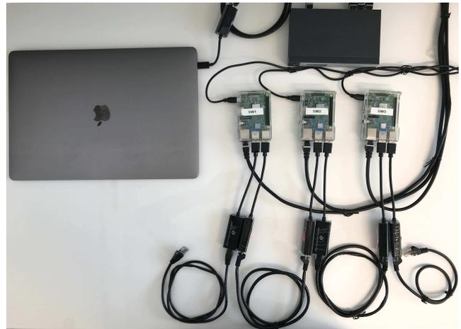
**Figure 3:** Our hardware SDN network is composed of three switches (i.e., Raspberry Pi 3 Model B) connected with each other through a linear topology, a controller (i.e., Apple MacBook Pro) and several hosts (not shown in the image) connected to the end of the Ethernet cables. All inter-switch and controller-switch links are 100 Mb/s.
